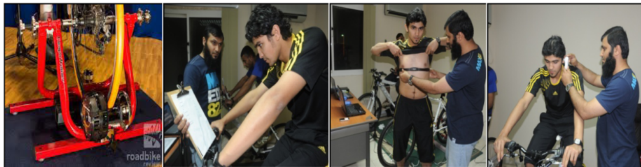
Fig. 3 This shows details of the experimental measurement of time trial, perceived exertion, heart rate and core temperature. The computrainer device is shown in the left panel. Details of the rate of perceived exertion scale (Borg's RPE 20-point Scale) and Polar Heart Rate Monitor are in the middle panel. The right panel shows a volunteer whilst their temperature is measured
